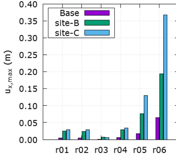
Figure 13: Maximum permanent horizontal displacements for seismic inputs a1–a4.
