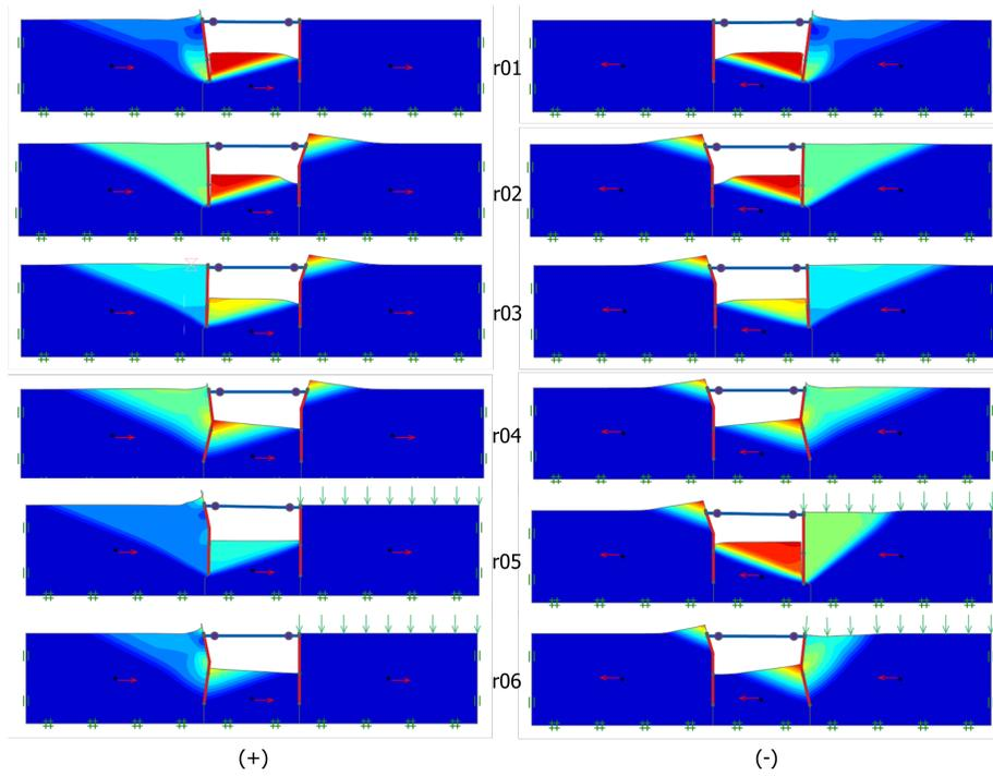
Figure 3: Contour maps of normalized velocity magnitude. Left column: positive pseudostatic force; right column: negative pseudostatic force.
