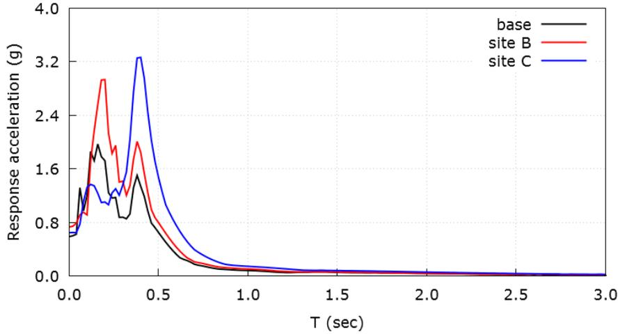
Figure 8: Response spectra for the seismic input at the base and for the accelerograms computed at a depth  $h$  for soil profiles B and C.
