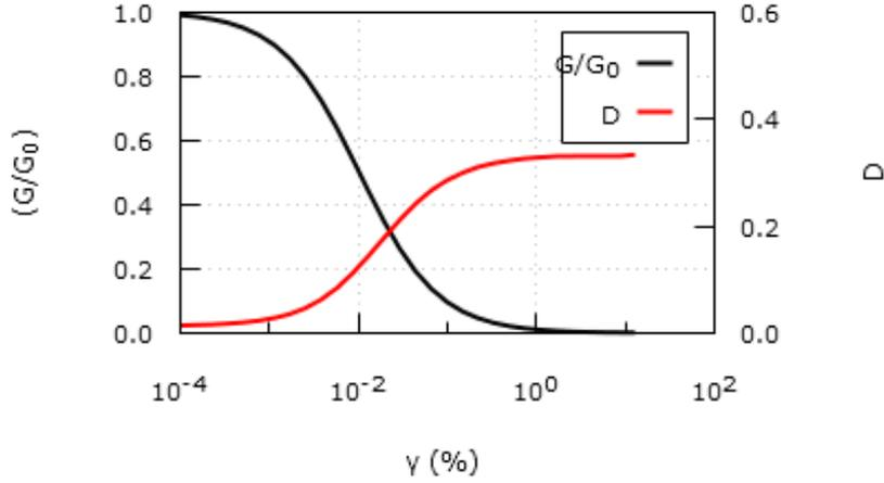
Figure 7: Shear stiffness decay curve (a) and damping ratio (b) *vs.* shear strain relation assumed in 1-d site response simulations.
