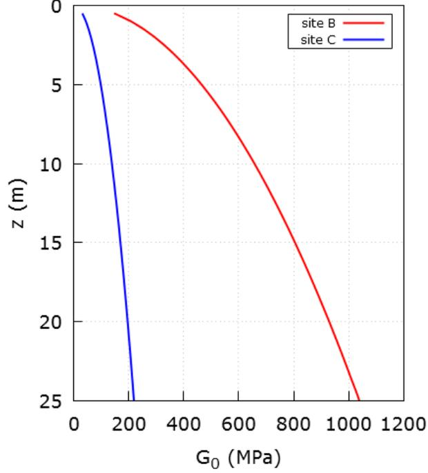
Figure 6: Profiles of small-strain shear modulus  $G_0$  assumed for soils type B and C.
