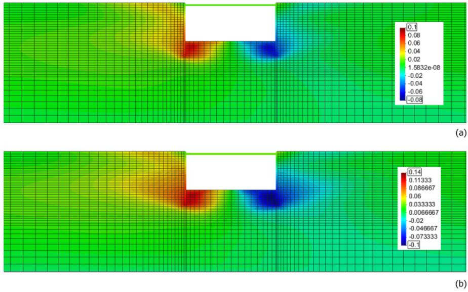
Figure 15: Contour maps of post-seismic horizontal displacement  $u_x$  computed by non-linear dynamic FE simulations: a) seismic input SI-1; b) seismic input SI-2.
