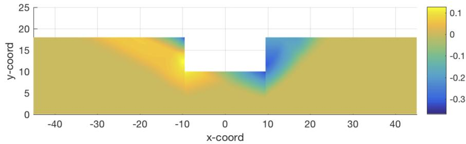
Figure 12: Simulation r06, soil profile C: contour maps of horizontal displacement  $u_x$ .
