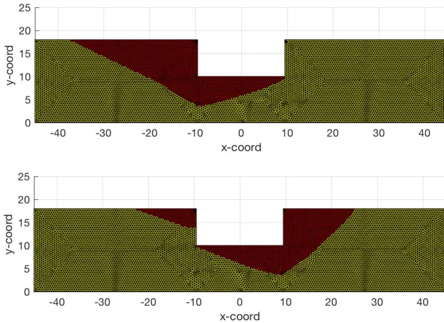
Figure 10: Simulation r06, soil profile C: plastic regions for the two collapse mechanisms.
