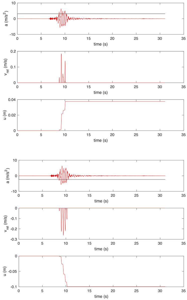
Figure 9: Simulation r06: Newmark integration for the two collapse mechanisms.
