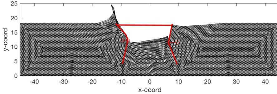
Figure 11: Simulation r06, soil profile C: deformed mesh for the combined displacement field.
