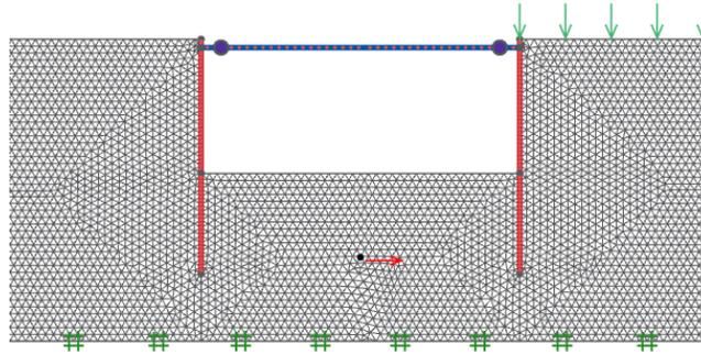
Figure 2: Detail of the FE-LA discretization of simulation r06, close to the excavation.
