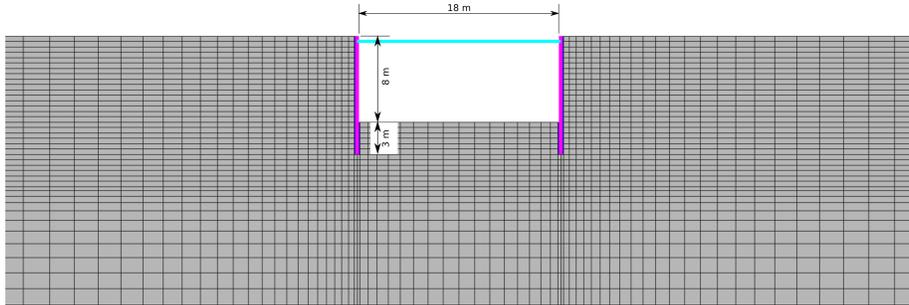
Figure 14: Detail of the discretization adopted in non-linear dynamic FE simulations (elements inside the excavation removed).
