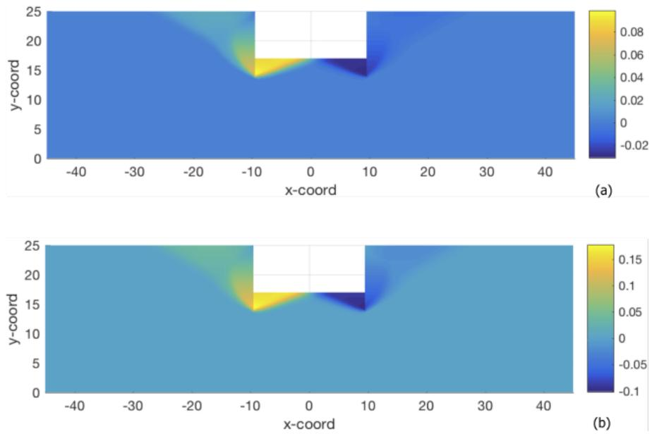
Figure 16: Contour maps of post-seismic permanent horizontal displacement  $u_x$  computed by the GNM: a) seismic input SI-1; b) seismic input SI-2.
