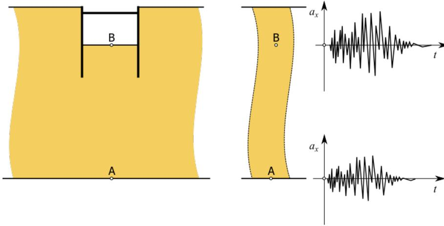
Figure 5: Definition of the seismic input via a 1-d site response analysis
