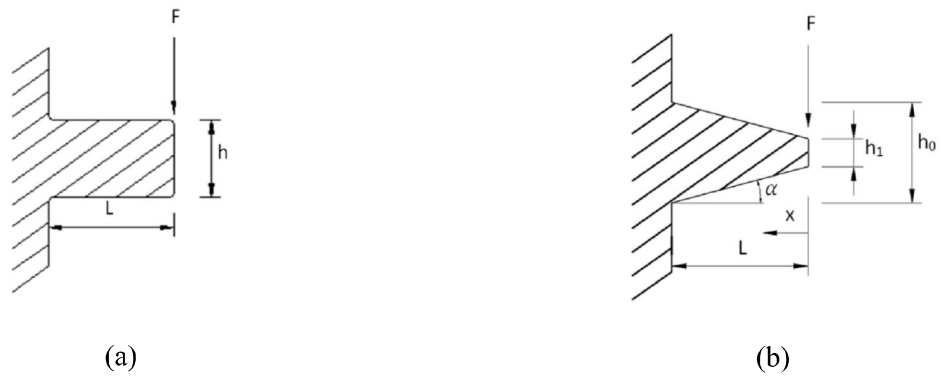
Figure 2. Thread shape: a) rectangular; b) trapezoidal.
