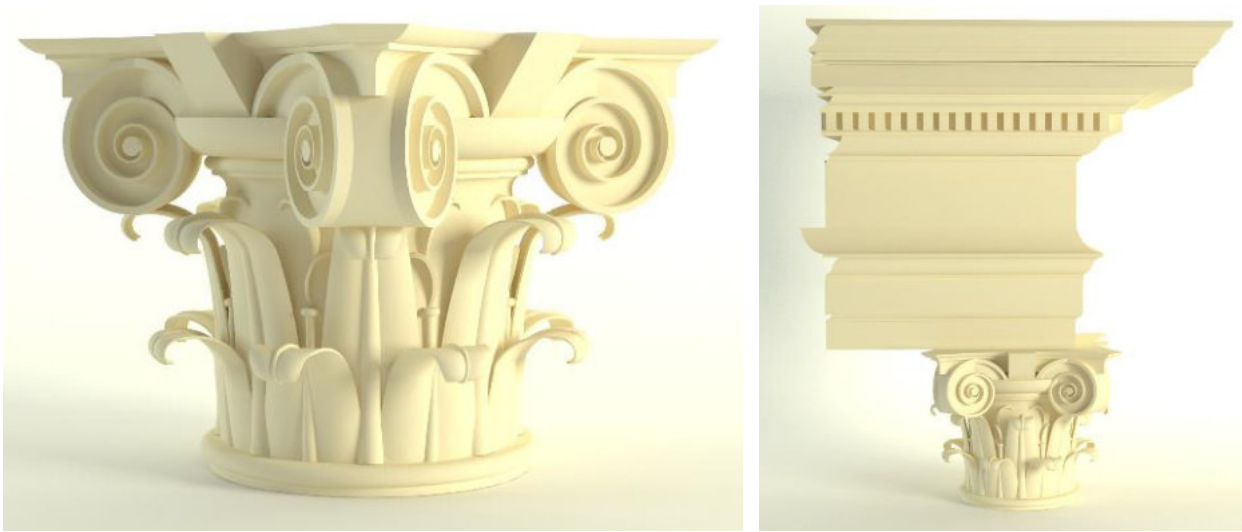
Fig. 4: Representation of the Corinthian capital and of its integration in the trabeation according to the Vignola interpretation
