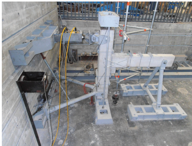
Figure 10: Picture of the experimental setup before the beginning of precast joint test.
