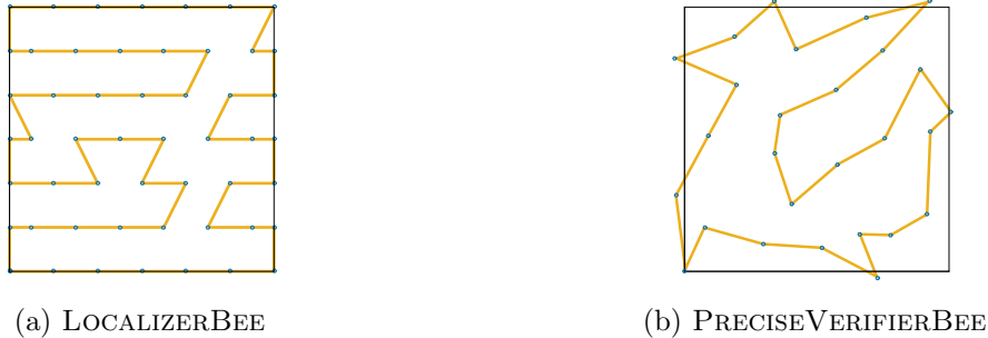
Figure 2: Example of LOCALIZERBEE and PRECISEVERIFIERBEE paths for drones
